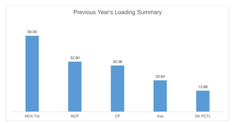
The Non-Coincident Peak Demand is 30.90 MW, which is around 60% of the total substation capacity of 50 MVA at a power factor of 0.96. The load factor or the ratio between the Average Load of 20.64 MW and the Non-Coincident Peak Demand is 60.75%. A safe estimate of the true minimum load is the fifth percentile load of 12.73 MW which is 42.10% of the Non-Coincident Peak Demand.
