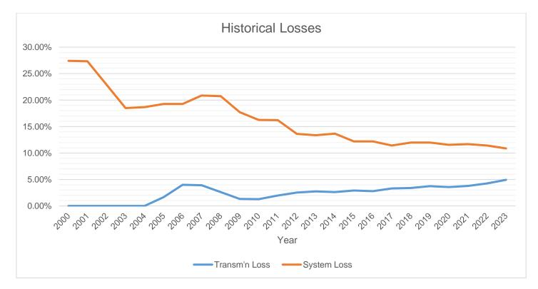
SORECO II's system loss, as seen in the above graph, has been improved dramatically for the last two decades. While transmission losses are kept at around 5%.
